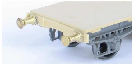
Because the flange at the base of each buffer projects above the headstocks, a small crescent shaped divot needs to be cut in each end at each buffer location with a 4mm chainsaw file. Each crescent should be about three boards wide and centred under the fourth board from each corner, but check the fit of the body against the underframe as work progresses.
