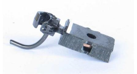
Cement the couplers to the underframe. Once the cement has hardened, use a 2.0mm drill to drill through the central hole in the coupler draft gear box and through the floor.
