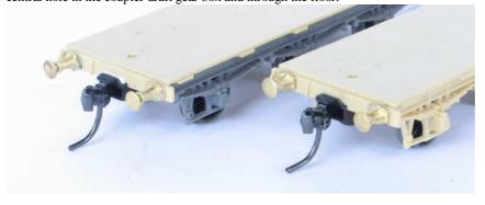
Now position the body on top of the underframe and use the 2.0mm drill to mark the position of the holes in the underside of the pieces of polystyrene glued in the body earlier. Drill 1.6mm holes on these marks and tap the holes M2. The body can be secured to the underframe with M2 x 8mm screws.
